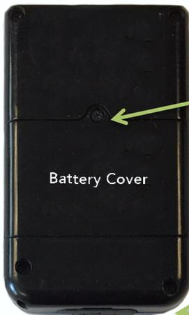
Remove the battery cover screw on the back of the KDC200/KDC250.KDC300. A longer screw will be included in your order.
