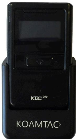
Insert the KDC into the adaptor, ensuring the USB connector is completely engaged in the USB port of the KDC. Once attached the screw hole on the back of the scanner should line up with the adaptor. Fasten the adaptor to the KDC with the supplied screw.
