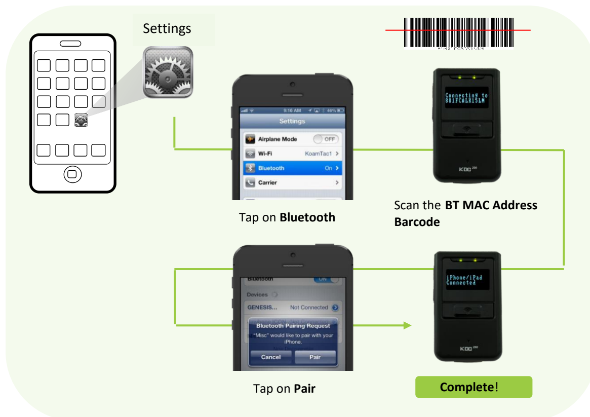
Figure 6 - Connecting KDC with a smart phone by scanning Bluetooth MAC Address Barcode
