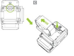
\*The replacement ringband description applies to both double ring scanners and ring scanners.
