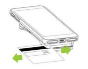
2. If the swipe is successful, you will hear a beep and the LED indicator on the right side of the device will flash green. If the swipe fails, the device will not beep and the LED indicator will flash red.
