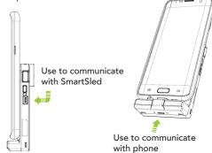
\*Both USB ports support KDC and phone simultaneous charging. GUA\_AM\_20230818
