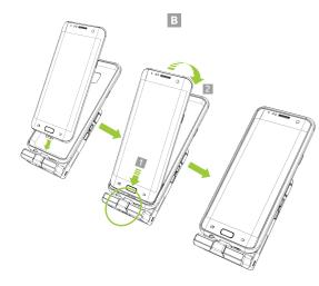
3. Inspect the connection between the General Universal SmartSled and previously installed USB Connect Head. To test the connection, attempt to charge your device via USB or Charging Cradle - a successful connection will indicate charging on your device.
