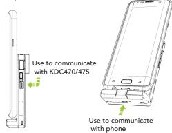
\*Both USB ports support KDC470/475/480/485 and phone simultaneous charging.
