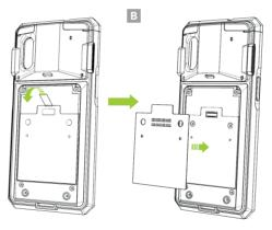
2. Remove the transparent protective film from the back of the companion cushion and attach it to the back of the SKX5 as shown below. (E)
