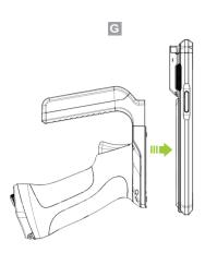
2. Insert the battery into the SKXSLED-UHF1.0W using the inner guide groove. (J)
