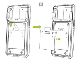
2. Remove the transparent protective film from the back of the companion cushion and attach it to the back of the SKX5 as shown below. (E)
