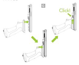
2. Insert the battery into the Pistol Grip. (J)
