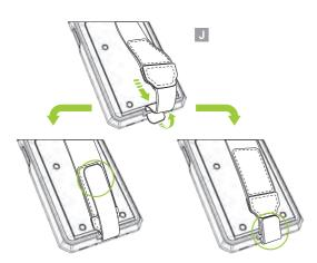
Flip the top cover back. After placing the sliding pad on the XCover screen as shown in the figure, remove the XCover by pushing up on the sliding pad with both thumbs. (H)
