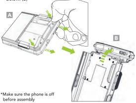
2. Slide the XCover smartphone into the SKX and flip the top cover forward as shown. (C)
