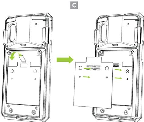
4. Remove the transparent protective tape from the back of the Companion Cushion and attach it to the back of SKXPro as shown below. (D)
