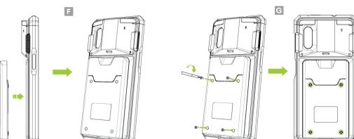
7. Using the screws removed in step 1, tighten the 0.5W UHF Companion to the SKXPro and replace the screw caps (G)
