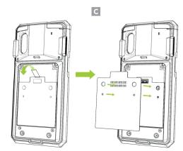
Remove the transparent protective tape from the back of the Companion Cushion and attach it to the back of SKXPro as shown below. (D)
