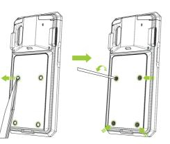
3. Attach the contact PCB to the SKXPro/SKX5. (C)
